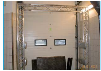
Stationary RFID gate at supplier Krause Meat
