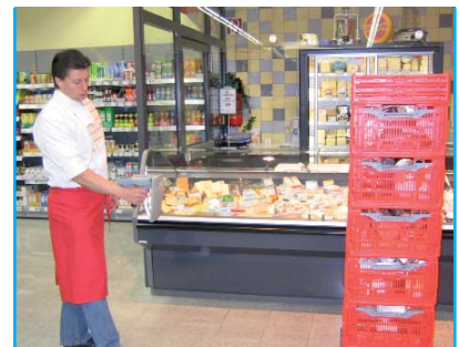
Reading the transponders with mobile RFID reader ("handheld") at grocery store
